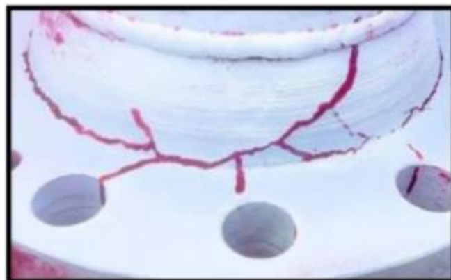
Figure 16: Dye used in penetrant should be good colour contrast against developer
