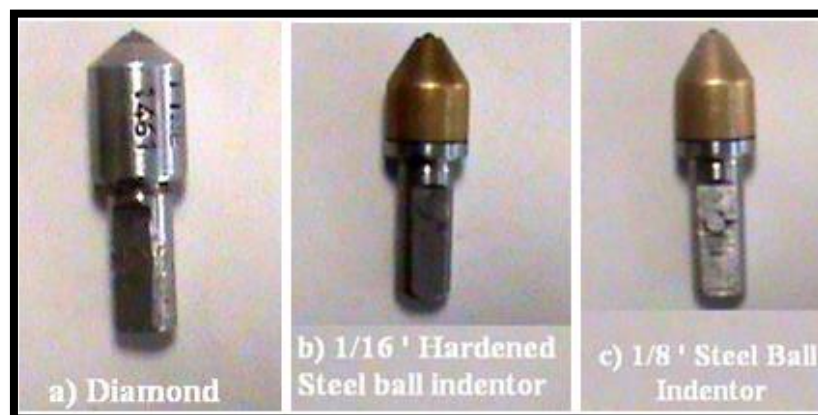
Figure 8: Indenter used namely mild steel, Brass, Aluminum as shown in Figure a, b & c
