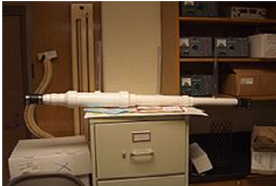
Fig. 2: Venturimeter - Experimental apparatus
