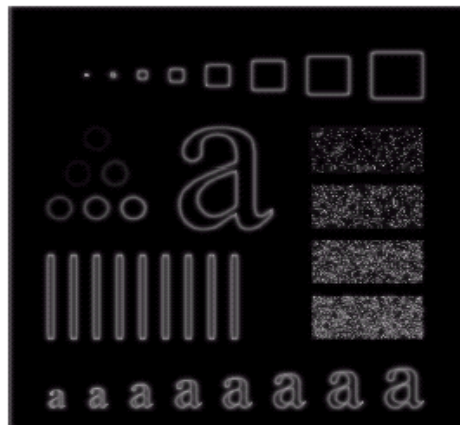
Results of Gaussian high pass filtering with D_0 = 30
