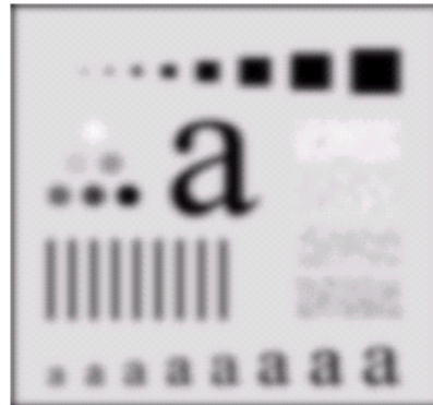
Result of filtering with Gaussian filter with cutoff radius 15
