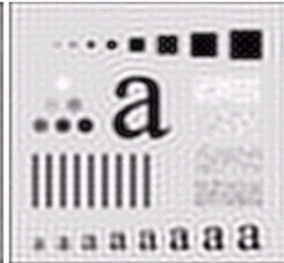
Result of filtering with ideal low pass filter of radius 30
