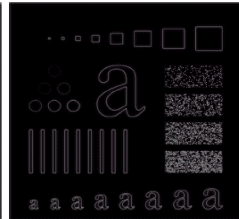
Results of Butterworth high pass filtering of order 2 with D_0 = 80
