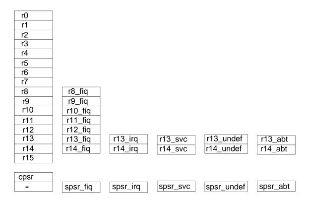
Every processor mode except user mode can change mode by writing directly to the mode bits of the cpsr. All processor modes except system mode have a set of associated banked registers that are subset of the main 16 registers. A banked register maps one-to-one onto a user mode register. If the processor mode is changed, a banked register from the new mode will replace an existing register.
