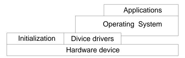
(i) The initialization code: It is the first code executed on the board and is specific to a particular target or group of targets. It sets up the minimum parts of the board before handling control over to the operating system. Initialization code (or boot code) takes the processor from the reset state to a state where the operating system can run. It usually configures the memory controller, processor caches and initializes some devices.
