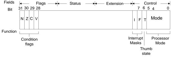
The cpsr is divided into four fields, each 8 bits wide: flags, status, extension and control. In current designs the extension and status fields are reserved for future use. The control field contains the processor mode, state and interrupts mask bits. The flag field contains the condition flags.
