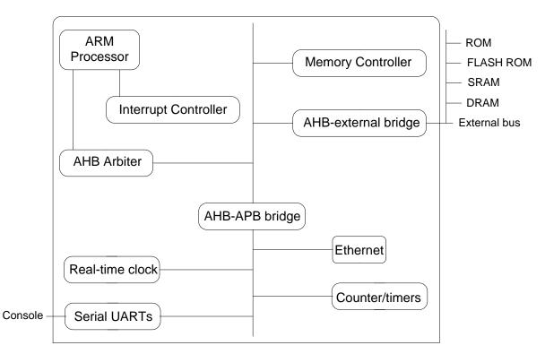
ARM processor based embedded system hardware can be separated into the following four main hardware components:
