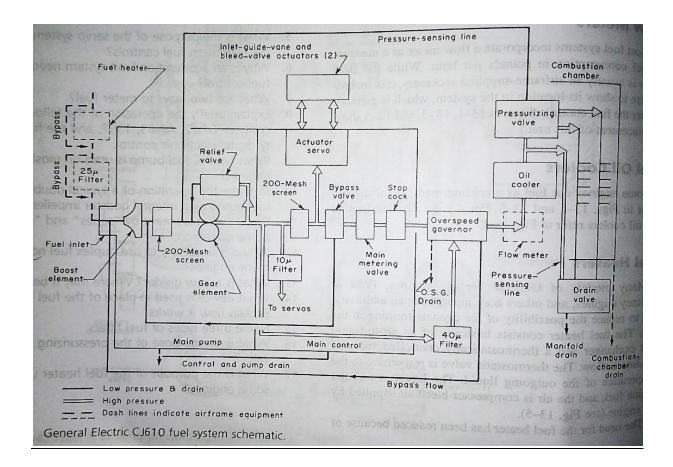
The CJ610 consists of the following engine mounted components:
