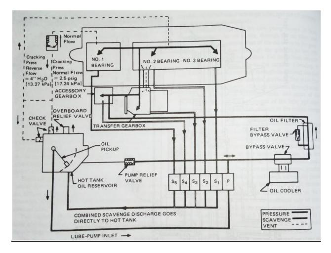
The oil-system component used on gas turbines is as follows:
