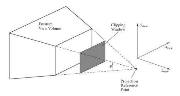
✓ For a given projection reference point and view-plane position, the field-of view angle determines the height of the clipping window from the right triangles in the diagram of Figure below, we see that
