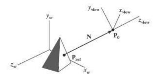
Specifying the view-plane normal vector N as the direction from a selected reference point  $P_{ref}$  to the viewing-coordinate origin  $P_0$ .
