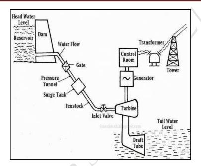
The hydroelectric power plant, also called as dam or hydro power plant, issued for generation of electricity from water on large scale basis. The dam is built across the large river that has sufficient quantity of water throughout the river. In certain cases where the river is very large, more than one dam can built across the river at different locations. The rain water flowing as river can be stored behind dams and released in a regulated way to generate hydro power.
