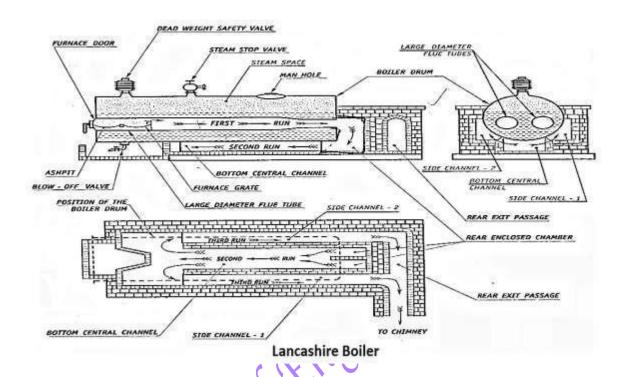
During the first, second and third pass the heat transfer takes place between hot flue gases and the water in the shell, converting water into steam.
