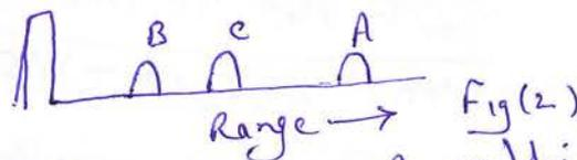
In above Fig. 1, Three targets A, B, C, where A within  $R_{unamb}$  and B and C are multiple-time-around targets.
